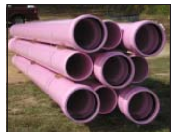
Contractors use "purple pipes" when installing a system for effluent water reuse. The pipes, valves, and outlets are color coded so utility personnel can easily identify what type of liquid is inside the pipe.
