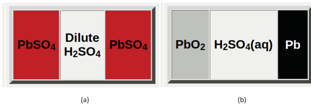
Figure 4. (a) Lead acid battery in fully discharged state; (b) fully charged state [3]
