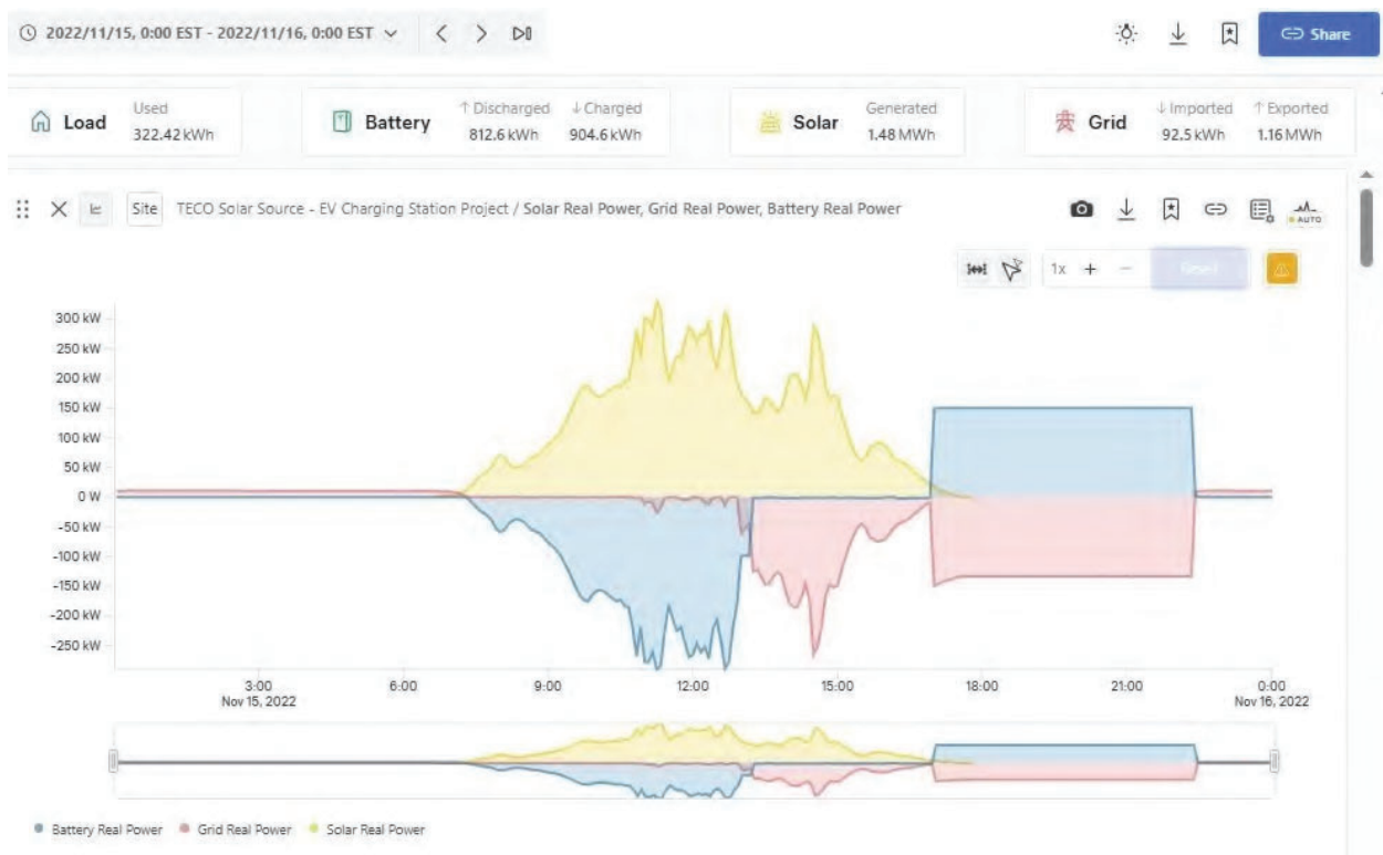
Figure 2 Battery Charge and Discharge Test 11/15/2022
