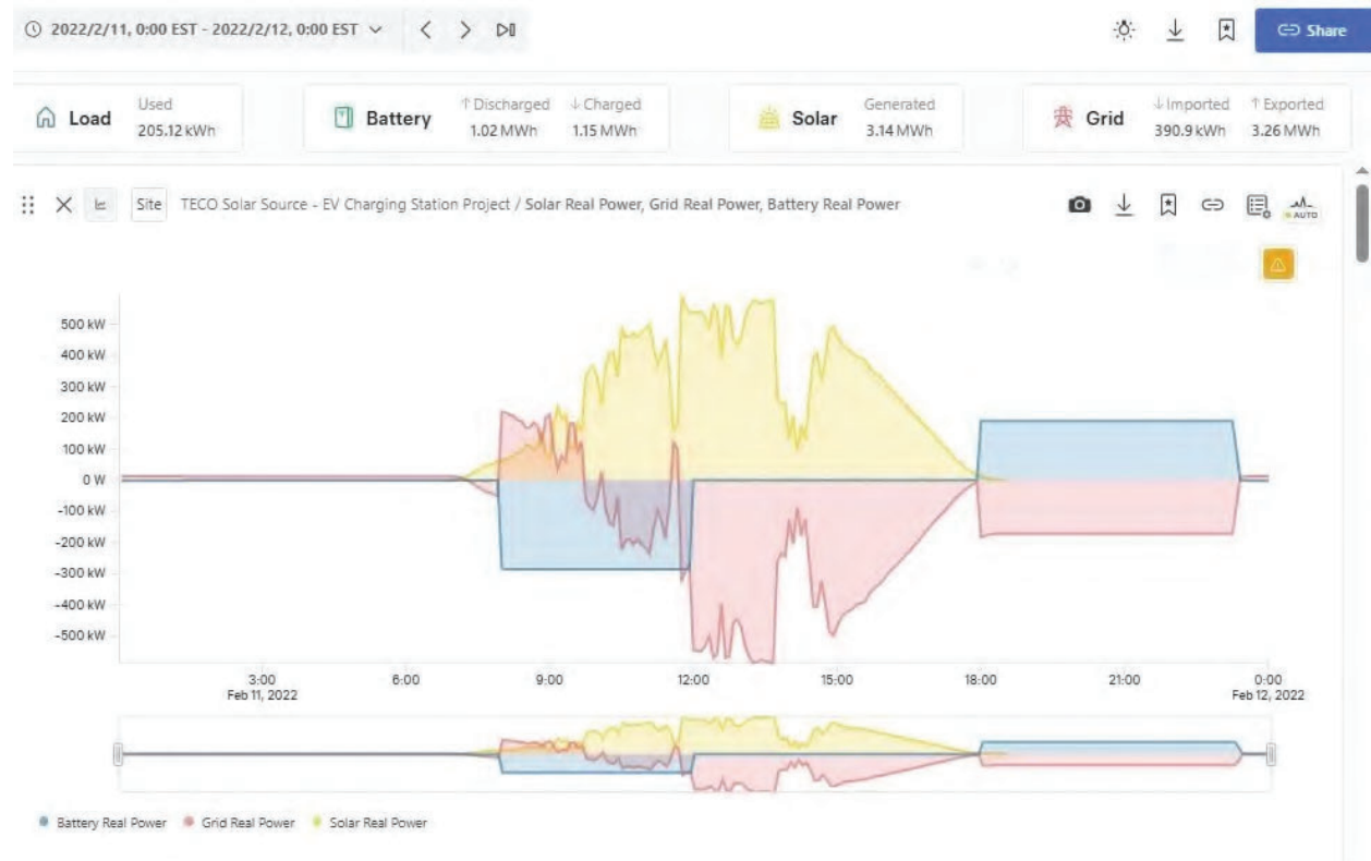
Figure 3 Battery Charge and Discharge Test 2/11/2022
