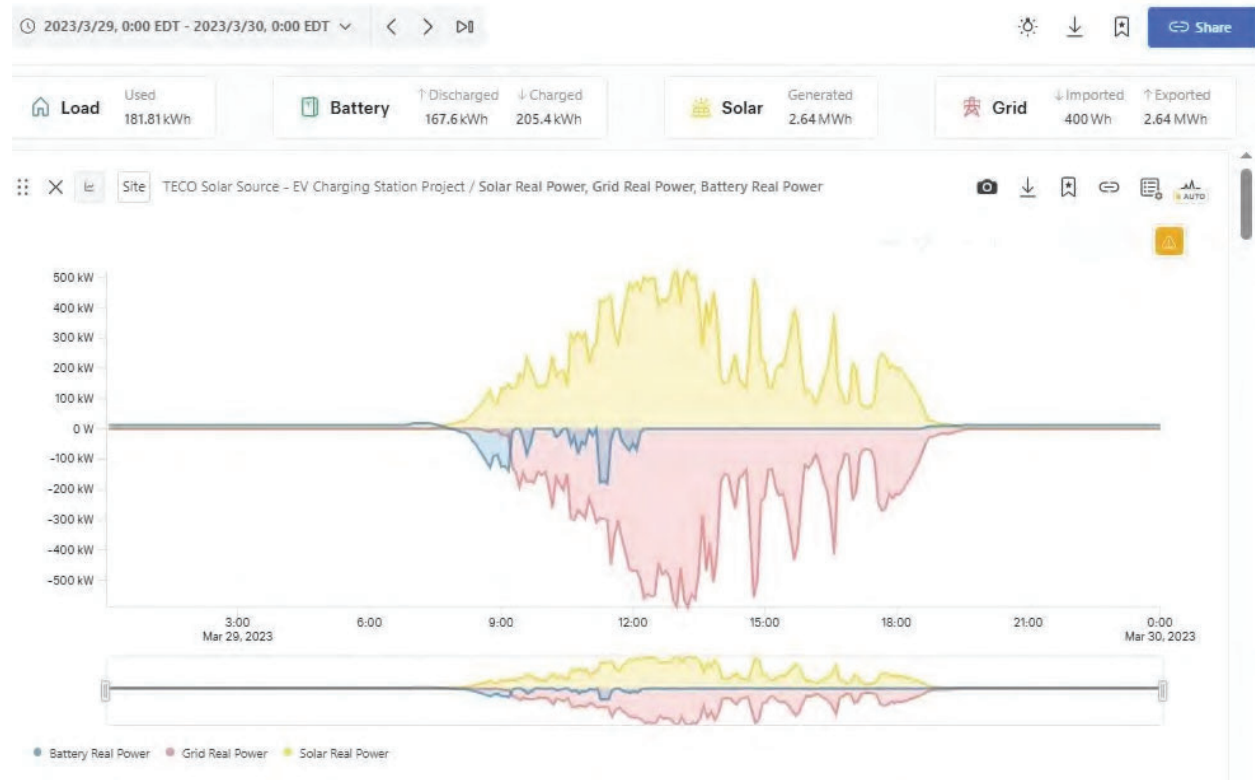
Figure 7 System Operation with No Battery Discharge to Grid 3/29/2023
