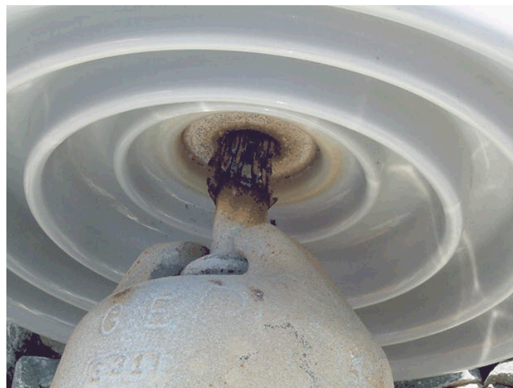
Typical Priority 1 "Ball & Socket" Insulator
