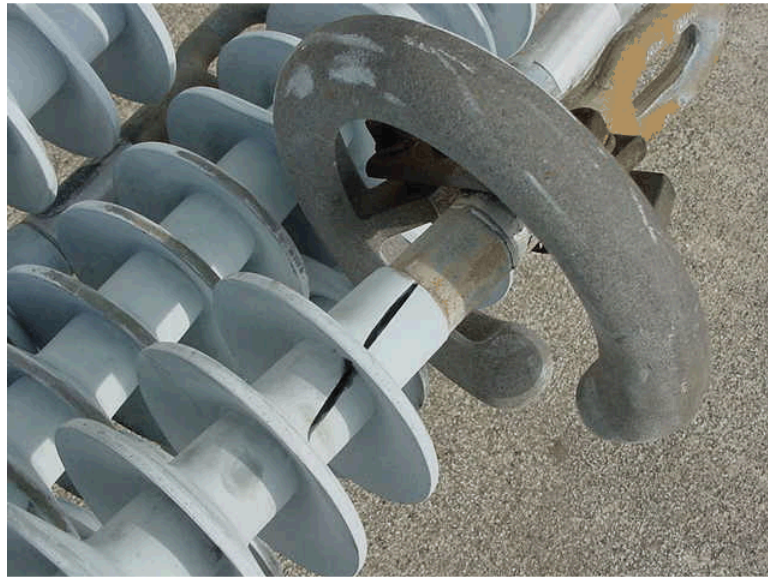
Priority 2 Polymer Insulator Split Housing (Ohio Brass)
