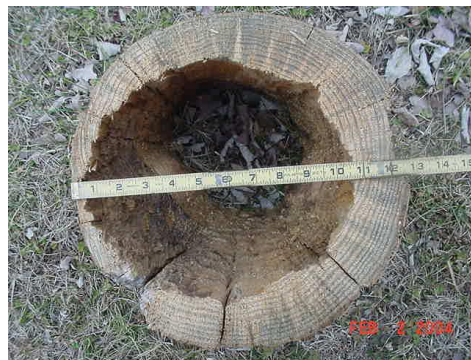
Priority 1 Internal Decay (Shell thickness less than 1 inch)
