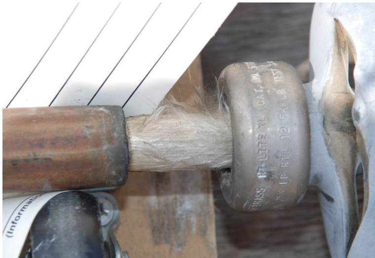
Priority 1 Polymer with exposed fiberglass rod
