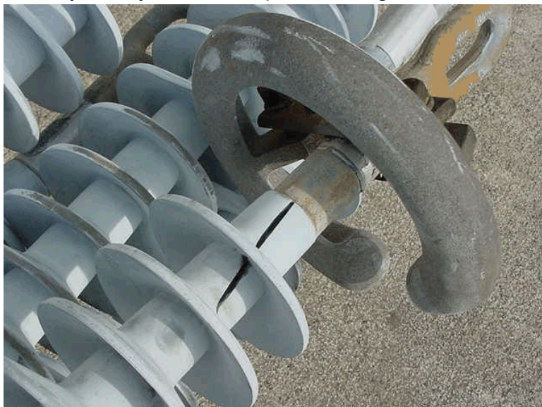
Priority 1 Polymer insulator with split housing.
