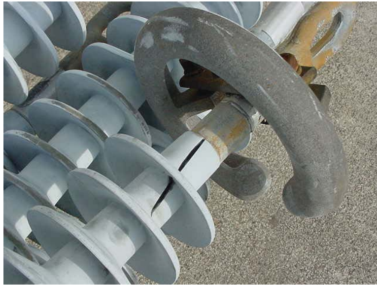
Priority 2 Polymer Insulator Split Housing (Ohio Brass)
