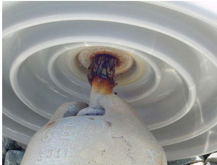
Typical Priority 1 "Ball & Socket" Insulator
