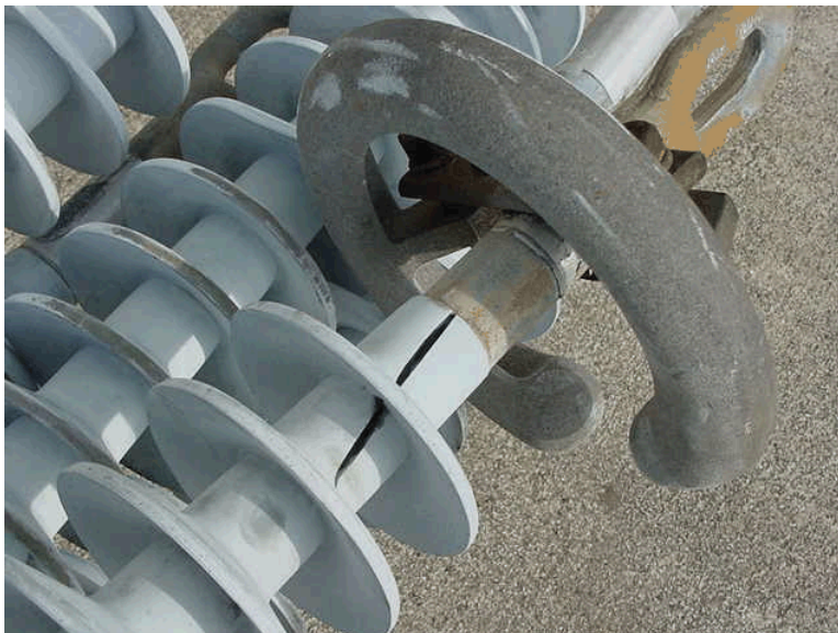
Priority 1 Polymer insulator with split housing.
