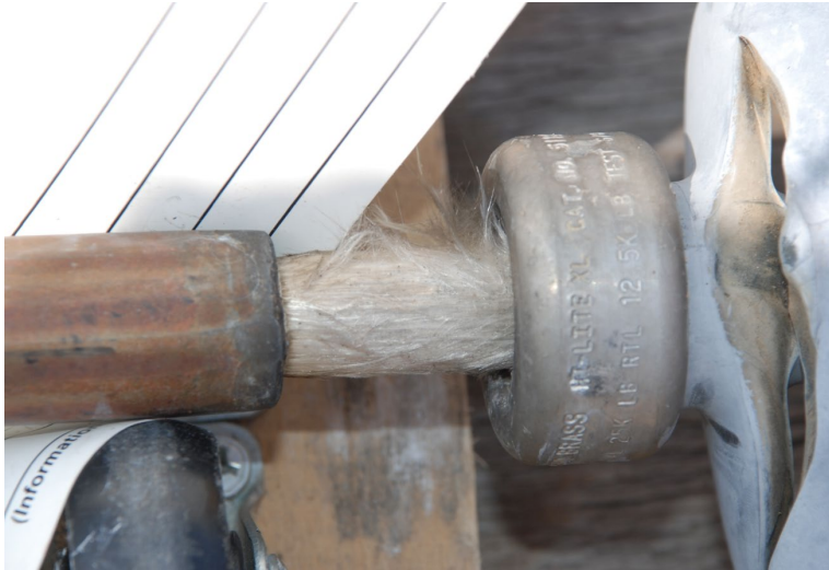
Priority 1 Polymer with exposed fiberglass rod.
